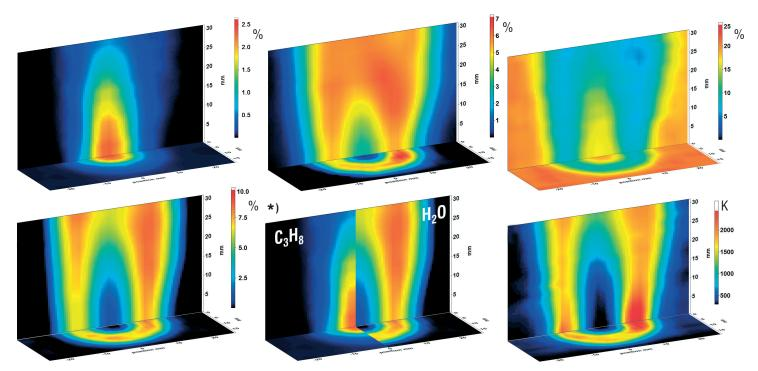
Axial and radial cuts of the propane-fueled Bunsen burner showing fuel  $(C_3H_8)$ ,  $CO_2$ ,  $O_2$ ,  $H_2O$  concentrations and flame temperature. The \*)-marked image presents the complementary fuel and water distribution.
