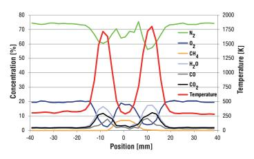
1D Raman imaging of gas composition and temperature in a propane-fueled Bunsen burner: spectrally seperated Raman lines and corresponding concentration (temperature) profiles.
