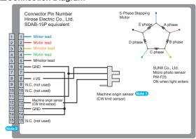
Note 1 When a travel command in the "+" direction is issued, the mounting table rotates to ∞ in the CCW (counterclockwise) direction viewed from the top surface, but it is stopped by the machine origin sensor (CW limit sensor) in the CW (clockwise) direction. Detect the machine origin using the method (MINI system) that detects the origin with a machine origin sensor (CW limit sensor).
